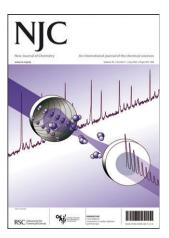
See Claire Vallance, page 867. A cavity ringdown spectrometer (shown schematically on the front cover) measures the time constant for the exponential intensity decay of light trapped within a two-mirror optical cavity. The time constant is strongly influenced by the presence of an absorbing species within the cavity, with the result that the technique allows absorption spectra to be measured with extremely high
